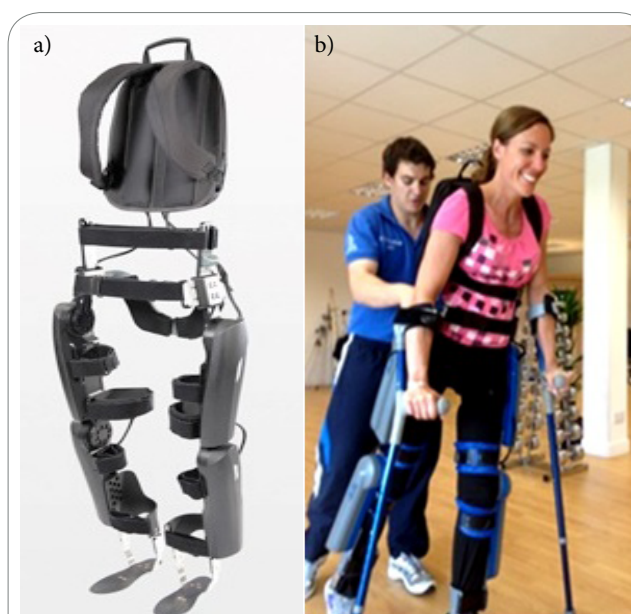
Figure 1: a) The ReWalk™ exoskeleton [23] and b) as used by a patient.
