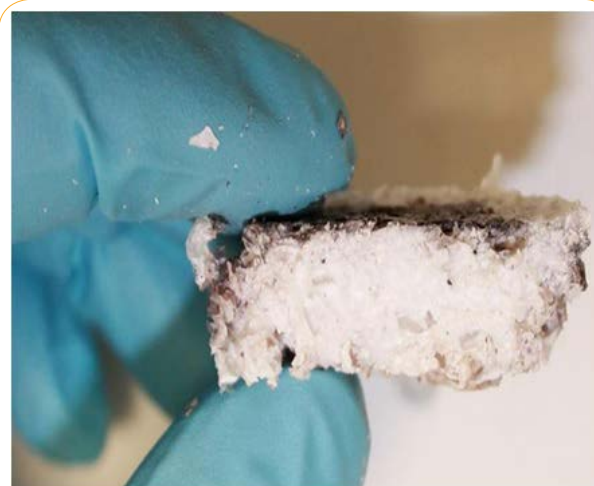
Figure 1: Cross-section of a porous PMMA-titania wafer fabricated with the benchmark method. The dark surface color is the result of photodeposited Ag when illuminated from above in aqueous AgNO 3 .
