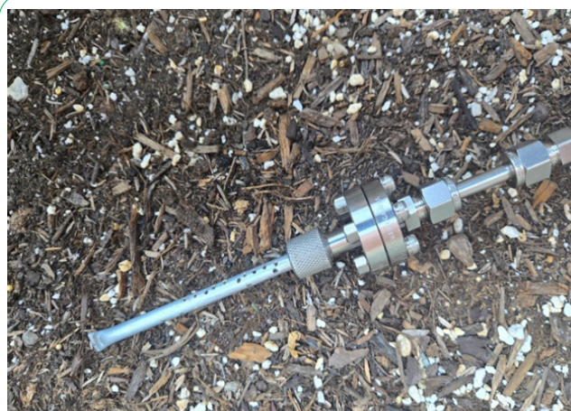
Figure 1: Photo of low volume soil probe prior to insertion into bare, unfertilized soil.
