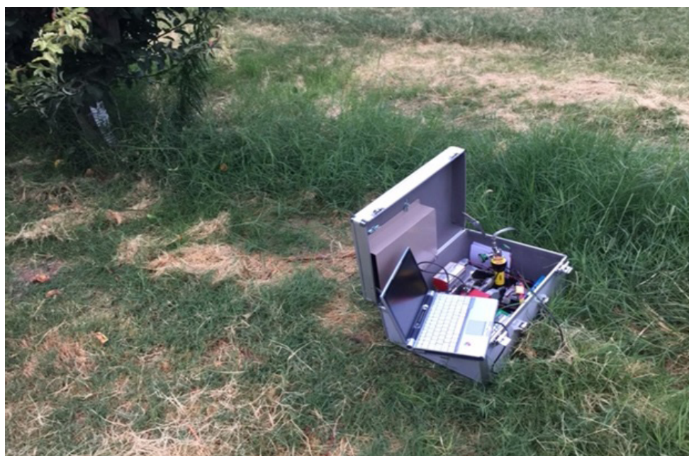
Figure 1: Photo of the quadrupole instrument in the apple orchard during measurements. The small inlet probe can be seen curved over the instrument case top side in the instrument case.
