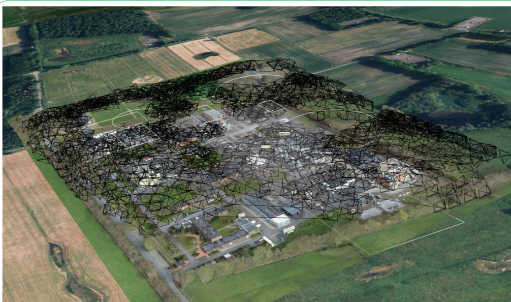
Figure 14: 3D flight planning taking into account infrastructure, risk and no-fly zones (Agisoft Metashape).
