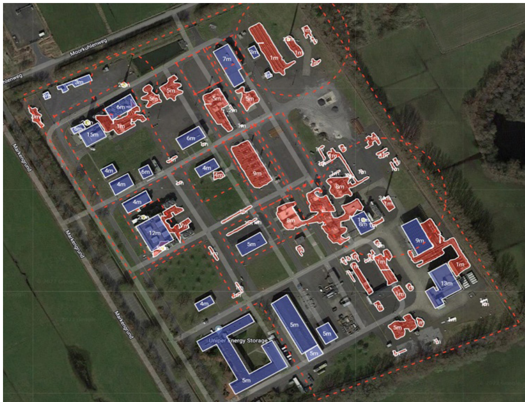
Figure 17: Validation of the 3D-Model by overlaying the processed 2D data.
