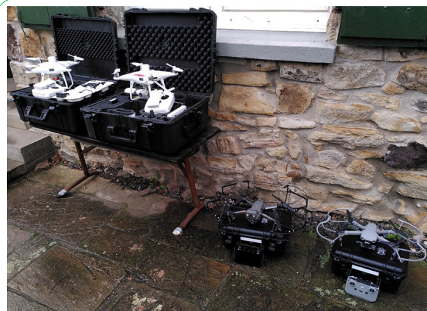
Figure 3: DJI UAVs with different sensors and capabilities used in the Research Center for surveying and geomonitoring purposes.
