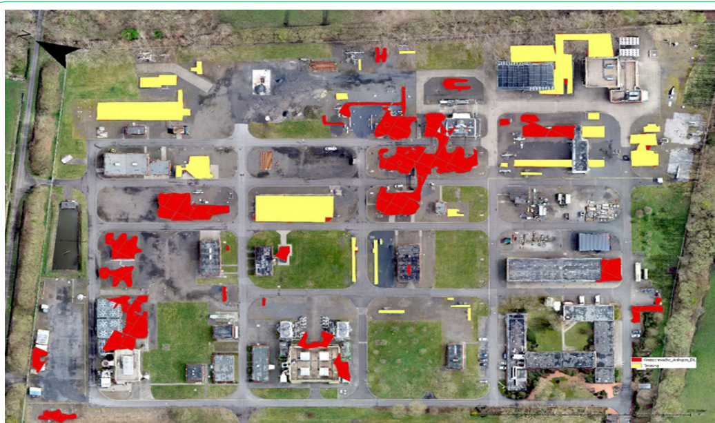
Figure 12: Detection of gas-technical equipment via Deep Learning in ArcGIS. Training objects are marked in yellow, detected objects in red.
