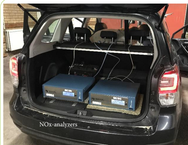
Figure 2: NO x -analysers hooked up to individual car batteries providing 24V DC.
