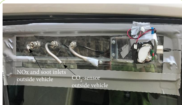
Figure 1: Outside vehicle inlets for NO x and soot, and one CO 2 -sensor mounted on the outside of the vehicle.
