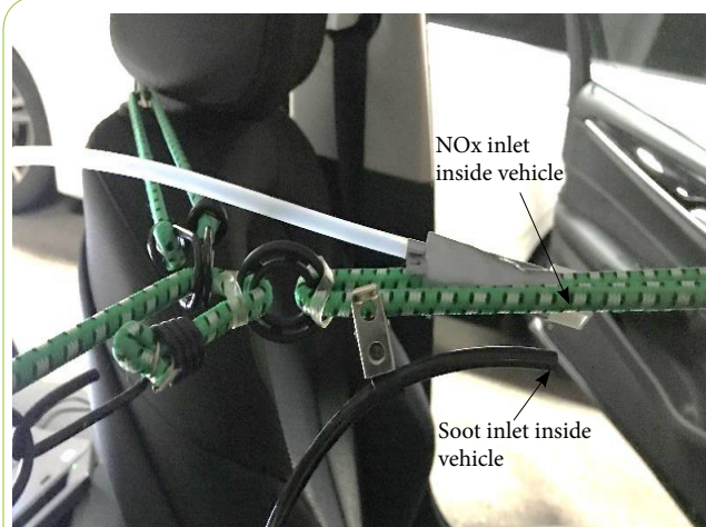
Figure 3: Inside vehicle inlets for NO x and soot, placed between driver seat and passenger seat.
