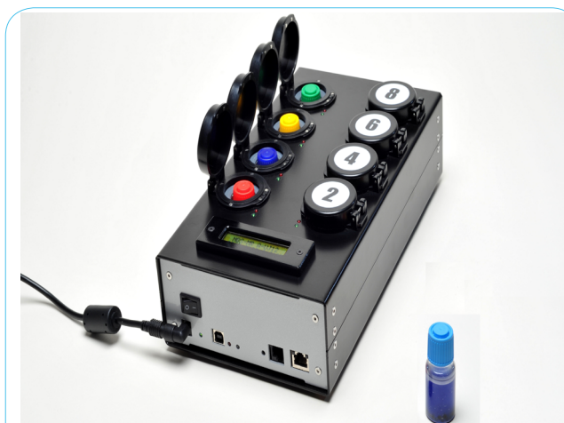
Figure 1: The MBS POCT device. The MBS POCT device is made of a ready-to-use disposable reaction vials (weight: 10 g; size: 60 mm height x 23mm diameter) and the MBS Multireader (weight: 1850 g; size: 315 x 175 x 95 mm).
